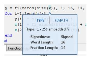
For a variable with a fixed-point type in the original code, when you place your cursor over the variable before or after conversion, the app displays the fixed-point type information.
