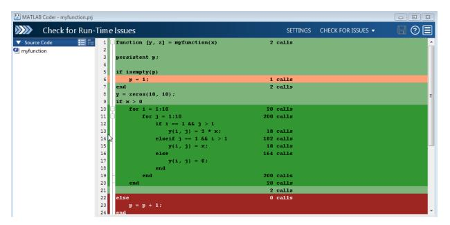
Line execution count collection is enabled by default. To disable the collection, clear the **Collect MATLAB line execution counts** check box. If line execution collection slows the run-time issue checking, consider disabling it.
